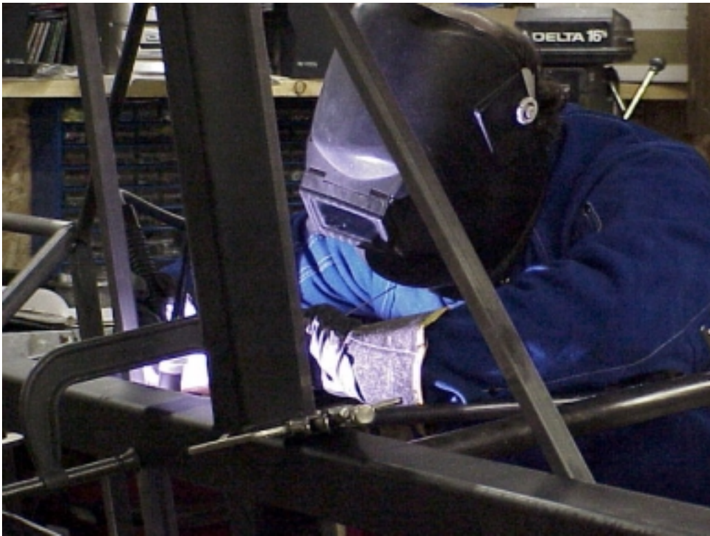
TIG (Tungsten Inert Gas) welding the prototype frame
