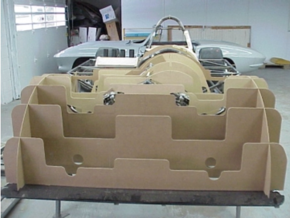
An engine was mocked up in foam for setting top deck clearances.
