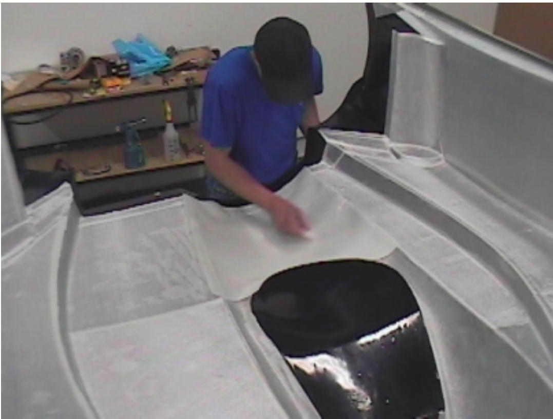
Advanced composite material being laid up in the mould. The next step is vacuum bagging and oven curing.
