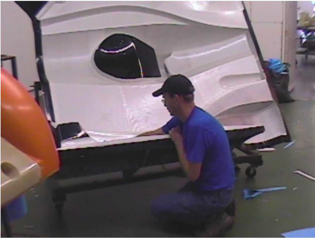
Advanced composite material being laid up in the mould. The next step is vacuum bagging and oven curing.
