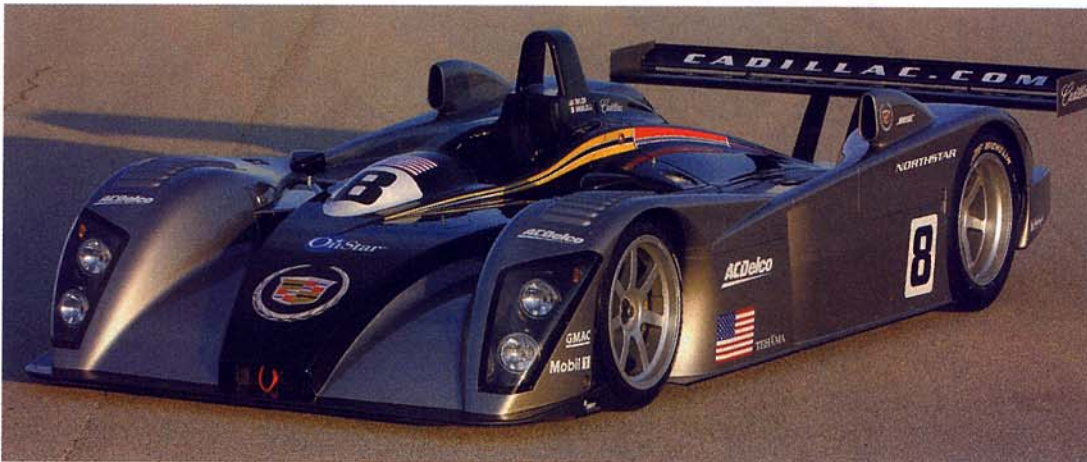
For the 2002 season, Cadillac introduced an all-new car featuring the minimalist bodywork philosophy employed by the top teams to minimize drag while contributing downforce.
