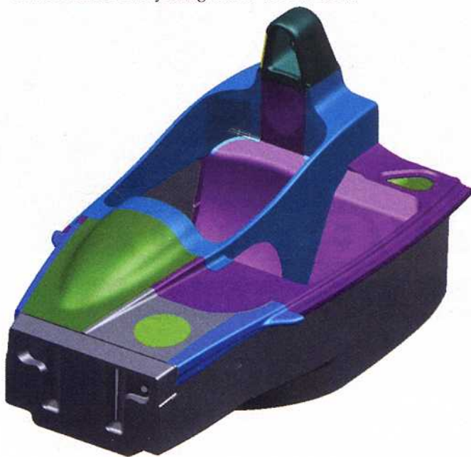
Each of the different colors represents different parts of the Cadillac's composite "tub" assembly. Notice how the gray wraps completely around the front of the chassis with no seams. Bonded to this main component are panels for the center spine, dash bulkhead, and additional strength in the area of the roll hoop.
