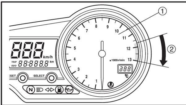
The electric tachometer allows the rider to monitor the engine speed and keep it within the ideal power range.
