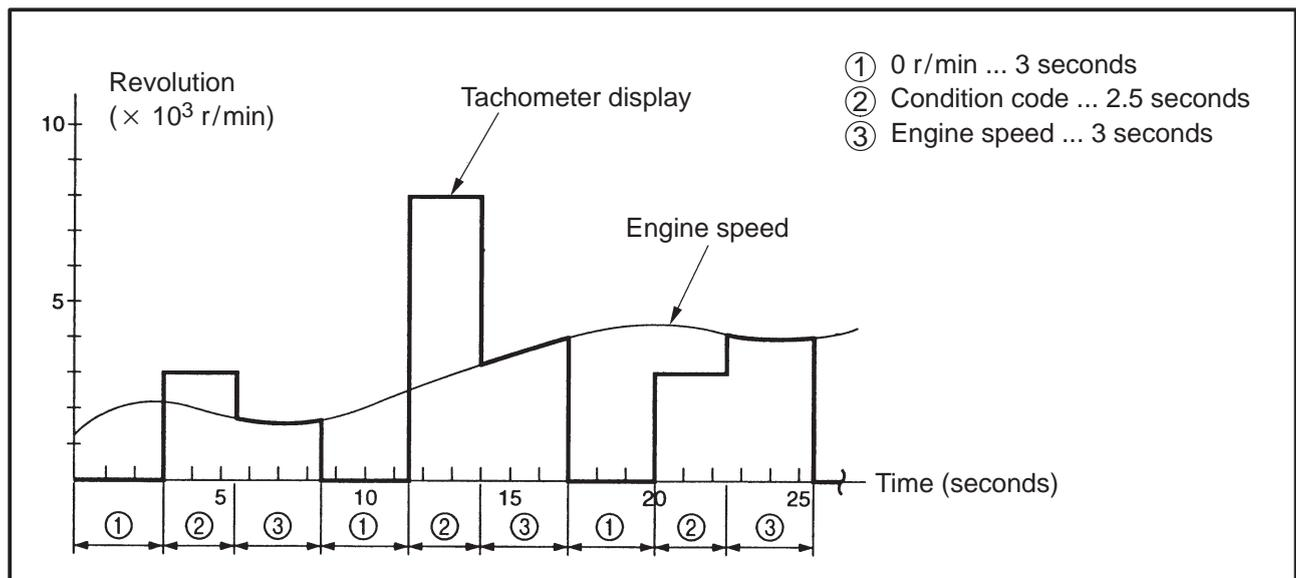
When more than one item is being monitored, the tachometer needle displays the condition codes in ascending order, cycling through the sequence repeatedly.
