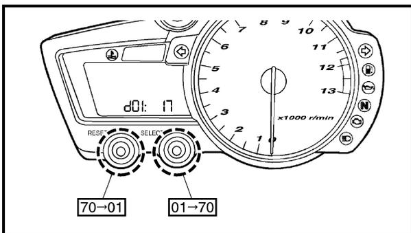
3. Using the "SELECT" button, select either the CO adjustment mode (which appears as "CO") or the diagnosis mode (which appears as "dIAG").
