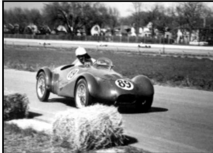
Sandy MacArthur brakes for a corner at the old Milwaukee Fairgrounds in the #89 Giaur. These cars vied with Bandini for the title of the lightest 750-engined car. The Giaur was built for the Italian Formula III class (750, not 500-cc). Twist a few Dzus fasteners and all the finders come off, making it a formula car.
